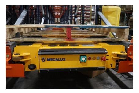
Controlled via a Wi-Fi-connected tablet, the pallet system places the load in the first available spot. This allows for easy picking and reduces the risk of damage and injury by not having the forklift drive into the raking.
