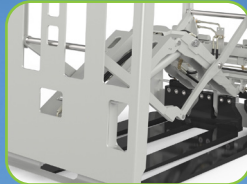
Adjustable outer platens to handle slipsheets
