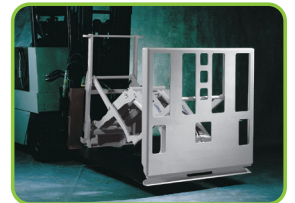
4. QFM Push/Pull is now ready for slipsheet loads.
