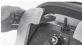
Move paddle backwards to go in reverse, frontwards to go forward; it could not be simpler or safer.
