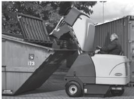
Variable dump height of up to 62 inches allows fast and simple disposal of swept debris.
