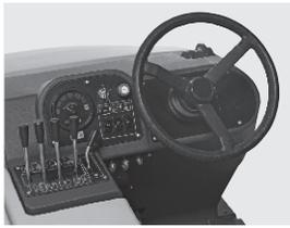
Ergonomic operator interface uses Analog-logic™ which allows a single operator motion to lower and activate the main broom and side brooms and open the hopper door.
