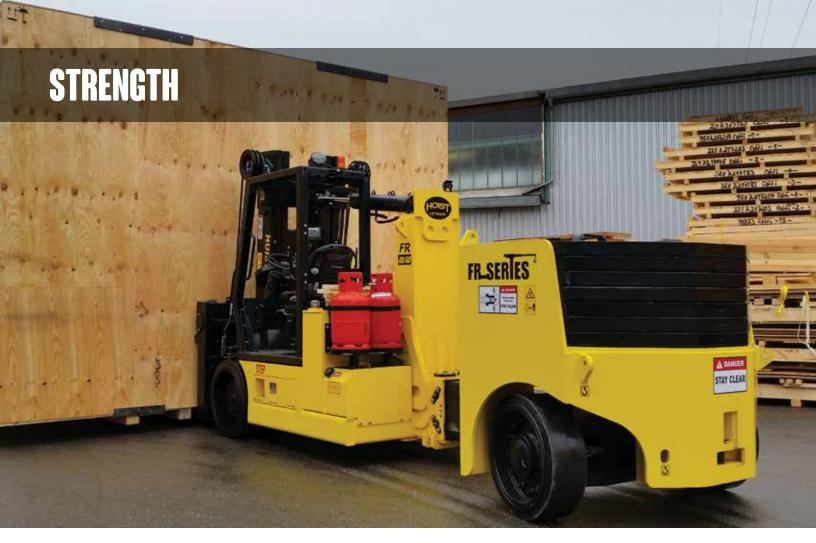
Hoist Liftruck's line of BIG TRUCKS starts with a strong foundation. The extendable chassis design of the FR Series provides excellent serviceability and versatility without sacrificing strength. The FR Series has been designed and tested to meet or exceed current, worldwide regulations for stability, sound levels and safety. Integrated lifting points also allow for safe handling and transport.
