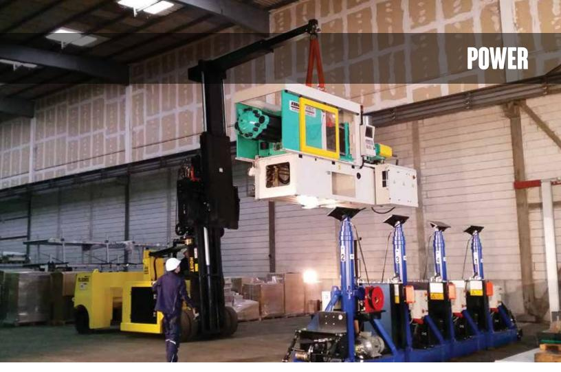
The FR Series is powered by a high-performance dual-fuel GM LPG engine and two-speed speed hydrostatic drive with variable RPM control. The "on-demand" hydrostatic drive pump offers not only power, but also increased productivity and fuel efficiency.
