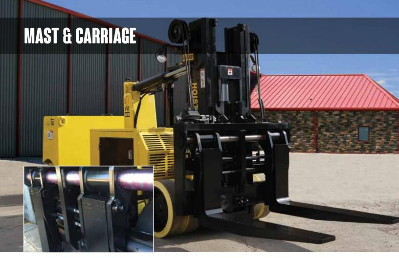
The FR Series comes equipped with a two-stage, free-lift mast and carriage with fork positioner. A hydraulically powered, multi-stage telescopic boom and collapsible stand come standard with most models (optional on FR 15/25).
